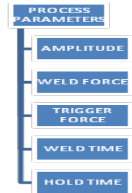
Fig. 2: Process parameter of Ultrasonic Welding
